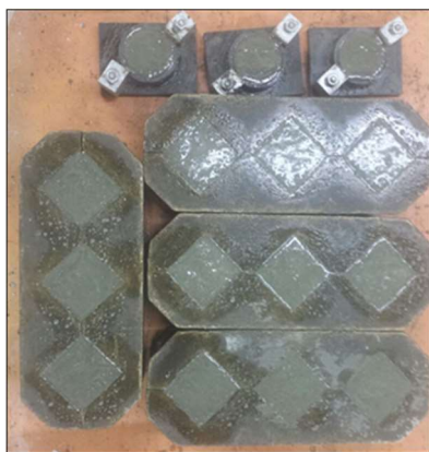
Figure 2: 50-mm cubes and thermal discs
